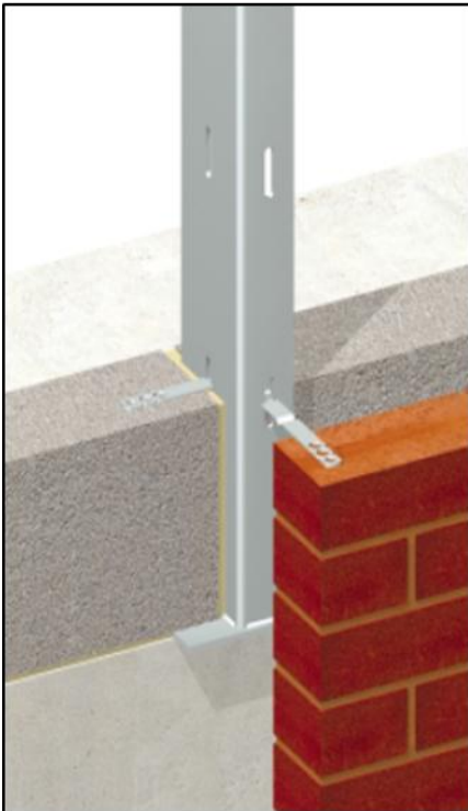
Typical arrangement for tying inner leaf of blockwork and outer leaf of brickwork to a windpost.
